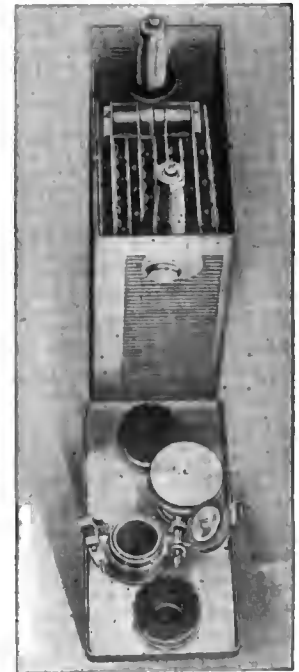
Fig. 6—Type A-4 cell, showing the positive and negative plates in the container, and also the removed cover with openings
